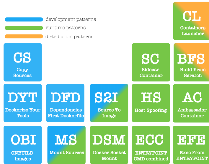
Figure 3.9: Visual representation of the container catalog of patterns from Lorio, organized into three color-coded categories: development, runtime, and distribution.
